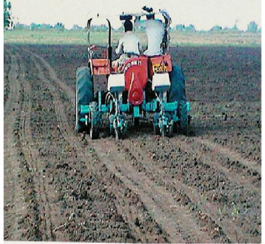
**Tractor operated cotton up rooter for removal of cotton stalks**
