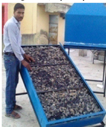
Fig. 2 Heat storage material loading in heat storage system of solar cabinet dryer
