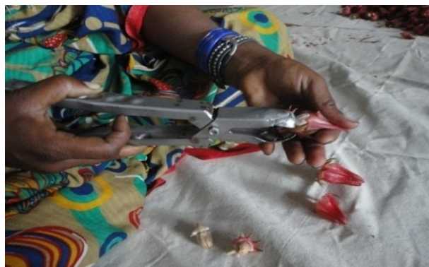
Plate 1 : Female labour detaching with Roselle Calyces Detacher
