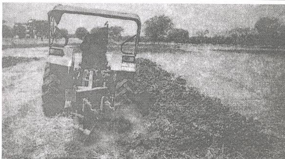
Fig3. Field testing of notched disc plough
